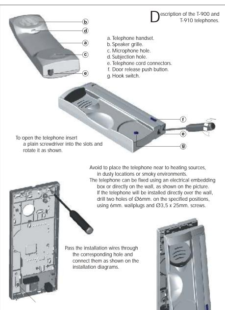
Close the telephone as shown on the picture. Once the telephone is closed, connect the handset using the telephone cord and put it on the craddle.
