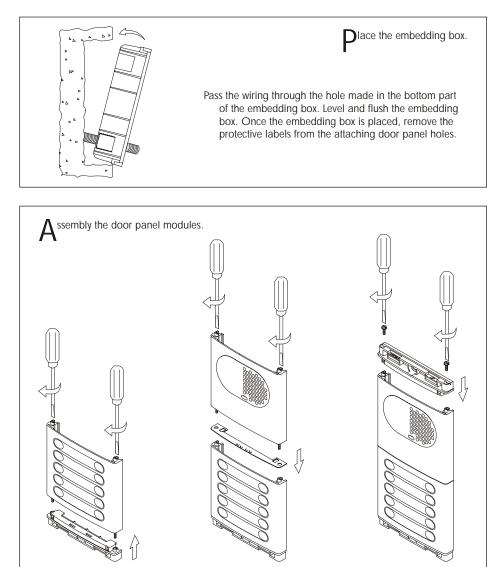
Insert the header DOWN marked in the lower module and fix it by screwing the module shafts.
