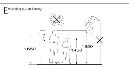
The upper part of the door panel should be placed at 1,65m. height roughly. The hole dimensions will depend on the number of door panel modules.
